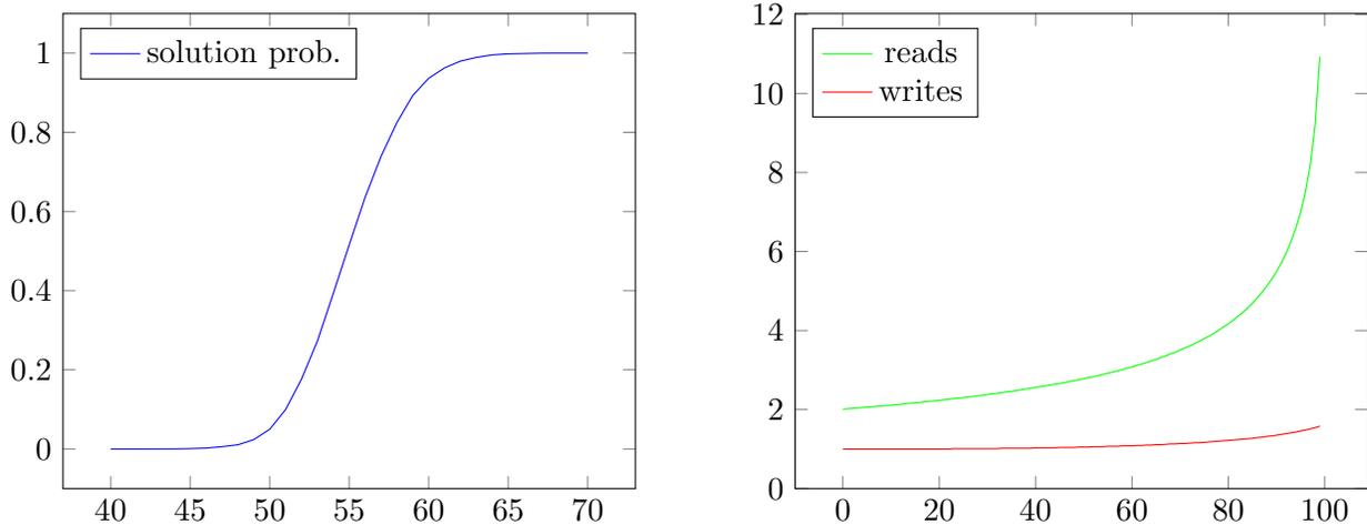
The left plot above shows the probability of finding a 42-cycle as a function of the percentage edges/nodes, while the right plot shows the average number of memory reads and writes per edge as a function of the percentage nonce/easiness (progress through main loop). Both were determined from 10000 runs at size  $2^{20}$ ; results at size  $2^{25}$  look almost identical. In total the program averages 3.3 reads and 1.75 writes per edge.
